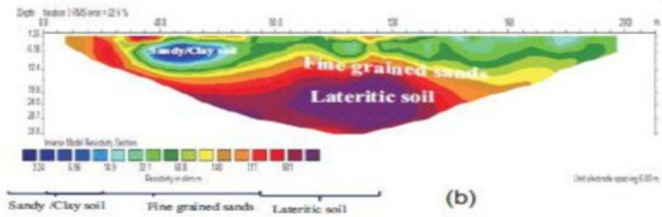
Figure 4.1b: Subsurface image obtained along ERT point 2 (Usung close, Oron L. G. A)
