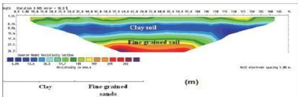
Fig.4.1m: Subsurface image obtained along ERT point 13 (Ikot Ebok, Eket L. G. A.)
