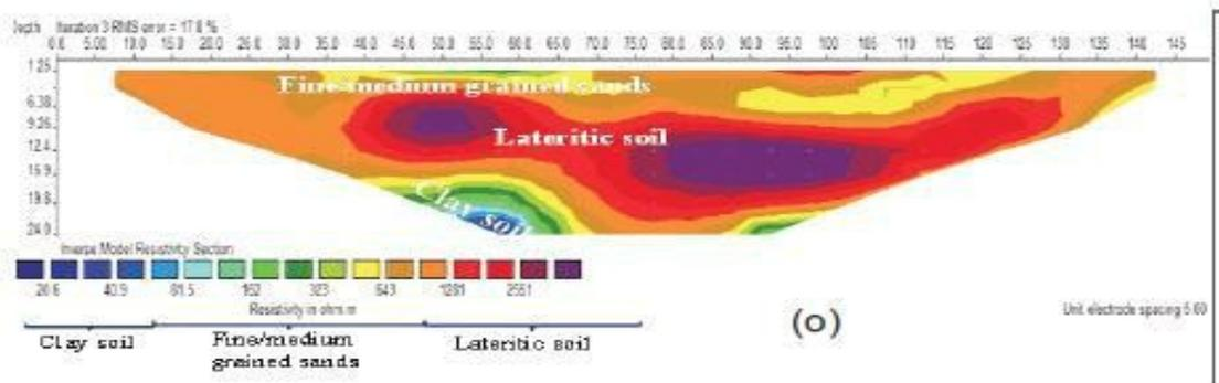
Fig.4.1o: Subsurface image obtained along ERT point 15 (Abighe Asang Uquo, Esit Eket L. G. A.)
