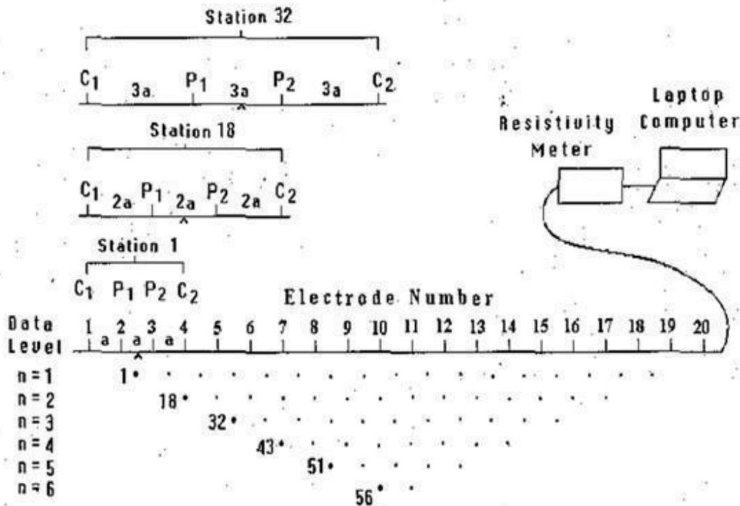
Fig.2: The arrangement of electrodes for 2-D electrical survey and the sequence of measurements used to build up a pseudo section (21)
