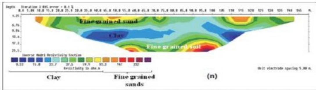
Fig.4.1n: Subsurface image obtained along ERT point 14 (Esit Urua, Eket L. G. A.)
