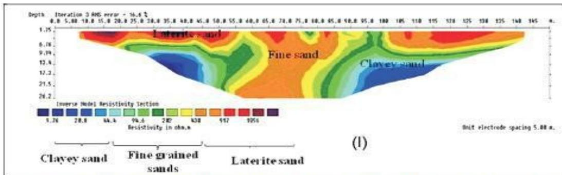
Fig.4.1l: Subsurface image obtained along ERT point 12 (Iko Town, Eastern Obolo L. G. A.)
