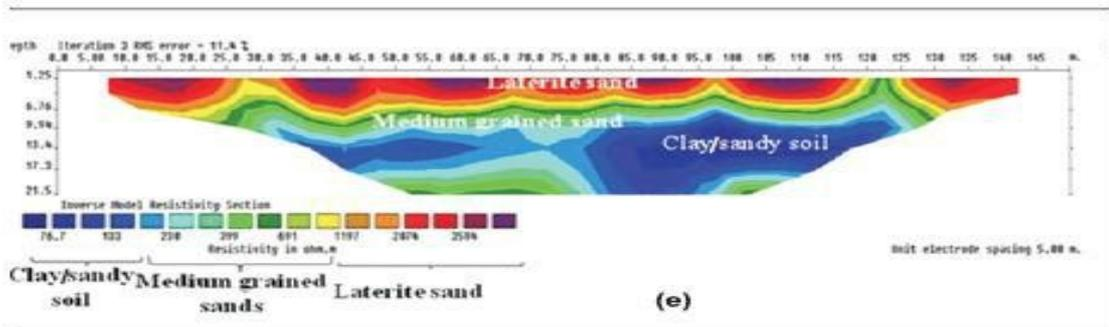
Fig.4.1e: Subsurface image obtained along ERT point 5 (Coconut Plantation, Ikot Akpaden, Mkpat Enin L. G. A.)
