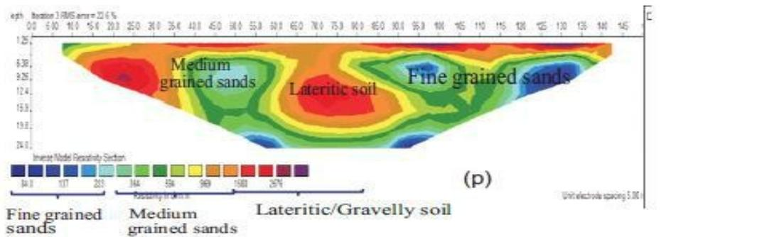
Fig.4.1p: Subsurface image obtained along ERT point 16 (Ikpa, Esit Eket L. G. A.)
