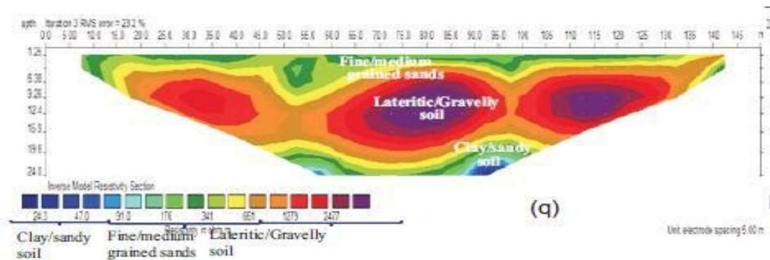
Fig.4.1q: Subsurface image obtained along ERT point 17 (Unyenghe, Mbo L. G. A.)
