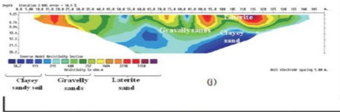
Fig.4.1j: Subsurface image obtained along ERT point 10 (Ette town along E-W road, Ikot Abasi L. G. A.)
