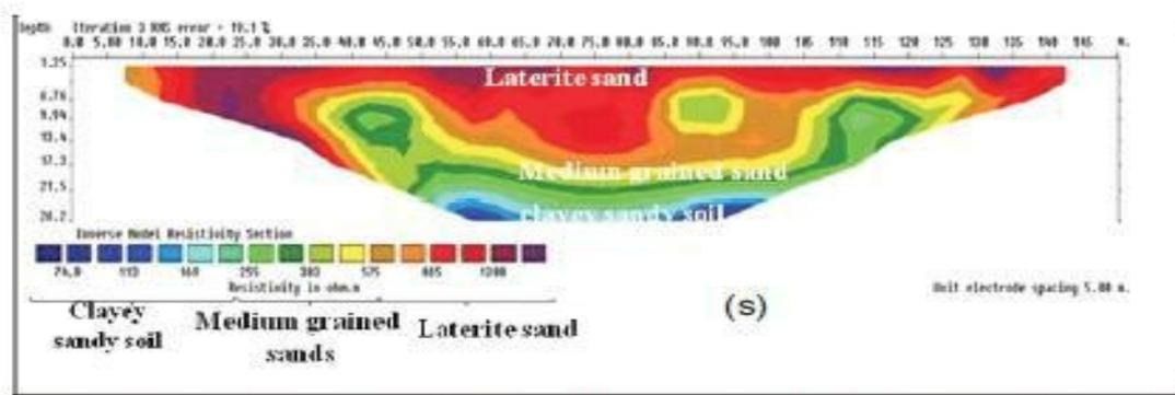
Fig.4.1s: Subsurface image obtained along ERT point 19 (Ibeno beach, Ibeno L. G. A)
